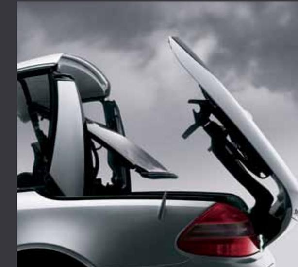
**Transforming.** The SL converts from secure hardtop coupe to freedom-loving open roadster in 16 seconds, using either a console-mounted switch or a button on the SmartKey remote. The rear window pivots 180° to help preserve usable trunk space with the top stowed.
