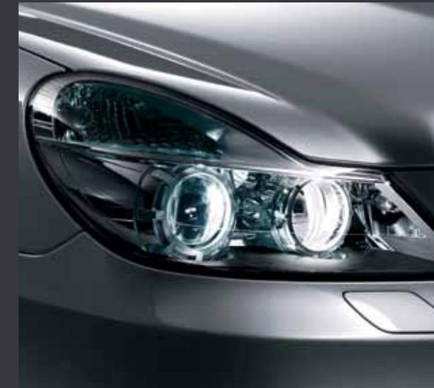
**Enlightening.** The SL's standard Bi-Xenon headlamps incorporate Active Curve Illumination, which swivels the beams according to your driving speed and steering angle. They increase usable illumination of curving roads by up to 90% over conventional fixed headlamps.
