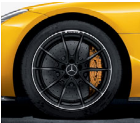
AMG 10-spoke forged wheels with 275/35 R 19 front and 325/30 R 20 rear tyres, painted matt black, rim flange with a high-shine finish (Code 658)
