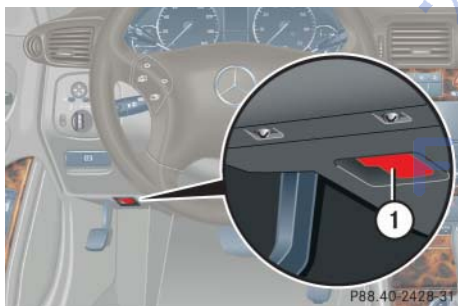
① Hood lock release lever
