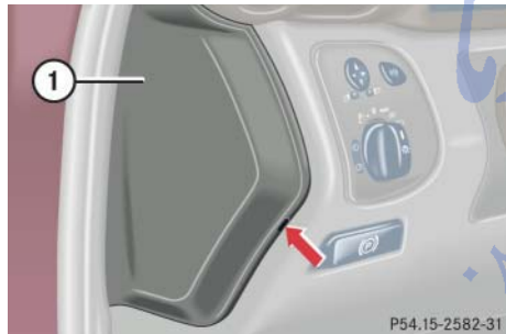
① Main fuse box cover
