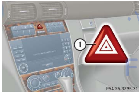
① Hazard warning flasher switch
