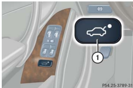
① Remote trunk opening switch with indicator lamp
