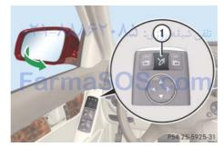
(1) Folds the exterior mirrors in and out
