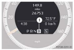
(1) Current gear selector lever position
