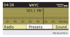
► Selecting "Radio" in the menu bar: Slide ← or rotate ( ).
