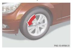
On wheel to be changed, loosen but do not yet remove the wheel bolts (approximately one full turn with wheel wrench).
