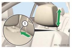
Head restraint height, manual adjusting
