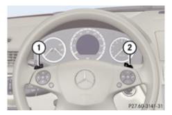
Steering wheel gearshift control (example illustration)
