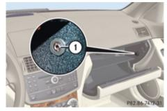
① AUX socket: Socket for 3.5 mm stereo jack, for devices with dedicated analog audio output or connection via headphone port, e. g. MP3 or tape player
