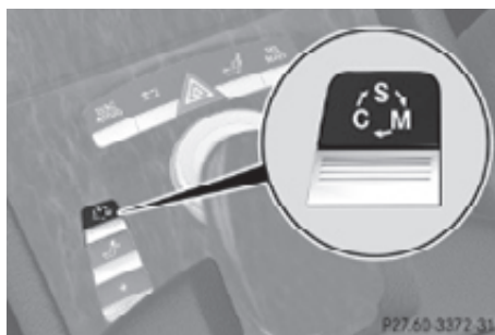
Program mode selector switch on AMG vehicles
