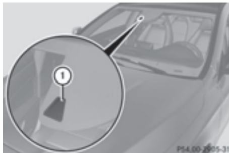
① Speed Limit Assist camera
