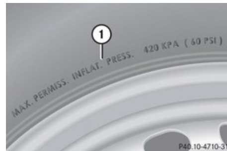
① Maximum permissible tire inflation pressure
