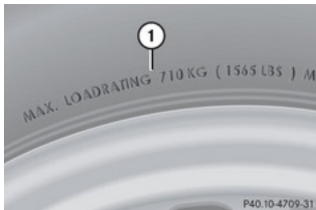
① Maximum tire load rating
