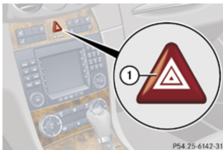
① Hazard warning flasher switch
