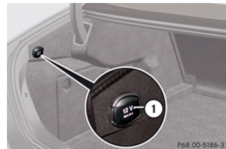
Power outlet in trunk
