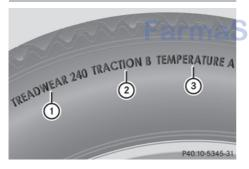
The Uniform Tire Quality Grading is a U.S. Government requirement. Their purpose is to provide drivers with consistent and reliable information regarding tire performance. Tire manufacturers are required to grade tires using three performance factors: tread wear (1), tire traction (2), and temperature resistance (3). Although not a Government of Canada requirement, all tires made for sale in
