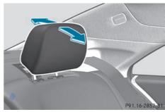
Pull or push the top of the head restraint until it is in the desired position.
