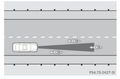
DISTRONIC PLUS has not yet detected the vehicle in front on the edge of the road,
