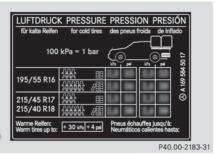
Tire pressure table with tire dimensions (example) Some tire pressure tables show only the rim diameters instead of the full tire size, e.g. **R18**. The rim diameter is part of the tire dimension and can be found on the sidewall of the tire (> page 332).
