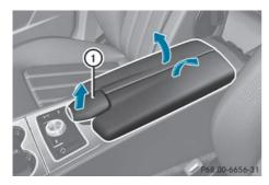
▶ To open: pull handle (1) upwards. The armrest folds out.
