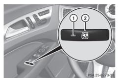
► To activate/deactivate: press button ②. If indicator lamp ① is lit, operation of the rear side windows is deactivated. Operation is only possible using the switches in the driver's door. If indicator lamp ① is off, operation is possible using the switches in the rear compartment.
