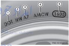
The TIN is a unique identification number. The TIN enables the tire manufacturers to inform purchasers of recalls and other safety-relevant matters. It makes it possible for the purchaser to easily identify the affected tires. The TIN is made up of manufacturer identification code (2), tire size (3), tire type
