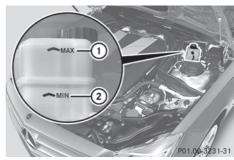
The brake fluid level is correct if it is between MIN marking ② and MAX marking ① on the brake fluid reservoir.
