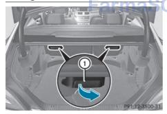
1 Vehicles with memory function: when you fold one or both parts of the rear seat backrest forwards, the respective front seat moves forward slightly, when necessary, in order to avoid contact.
