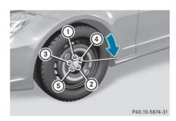
➤ Tighten the wheel bolts evenly in a crosswise pattern in the sequence indicated (① to ⑤). The tightening torque must be 96 lb-ft (130 Nm).
