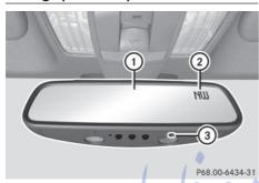
To obtain a correct display in rear-view mirror ①, the compass must be calibrated and the magnetic field zone must be set.
