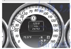
When DISTRONIC PLUS is activated, one or two segments ② in the set speed range light up.
