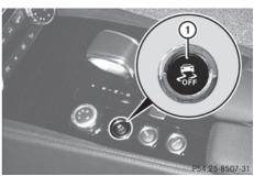
► To deactivate: press button ① until the ESP® OFF warning lamp lights up in the instrument cluster.
