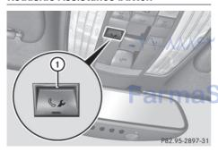
▶ Press and hold Roadside Assistance button ① for more than two seconds. This initiates a call to the Mercedes-Benz Customer Assistance Center. The indicator lamp in Roadside Assistance button ① flashes while the call is active. The Connecting Call message appears in the multifunction display. The audio output is muted.
