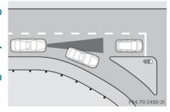
DISTRONIC PLUS does not brake for obstacles or stationary vehicles. If, for example, the detected vehicle turns a corner and reveals an obstacle or stationary vehicle, DISTRONIC PLUS will not brake for these.
