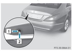
► Turn the mechanical key counter-clockwise from position 1 as far as it will go to position 2.
