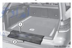
The EASY-PACK rear sill protector is attached to the underside of the EASY-PACK folding cargo compartment floor by means of magnets. It is designed to prevent clothing becoming stained and the paintwork being scratched when loading.
