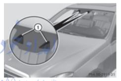
Lane Keeping Assist monitors the area in front of your vehicle with camera (1), which is mounted at the top of the windshield. Active Lane Keeping Assist detects lane markings on the road and can warn you before you leave your lane unintentionally.
