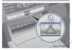
► To switch on the hazard warning lamps: press button ①.
