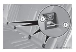
When installing the LATCH-type (ISOFIX) child restraint system, fold protective caps (2) of LATCH-type (ISOFIX) securing rings (1) inwards.
