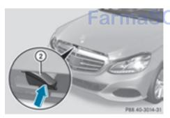
▶ Reach into the gap, pull hood catch handle (2) up and lift the hood. If you lift the hood by approximately 15 in (40 cm), the hood is opened and held open automatically by the gas-filled strut.
