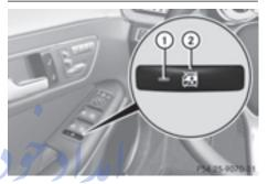
▶ To activate/deactivate: press button ②. If indicator lamp (1) is lit, operation of the rear side windows is disabled. Operation is only possible using the switches in the driver's door. If indicator lamp (1) is off, operation is possible using the switches in the rear compartment.
