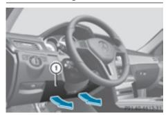
Driver's knee bag (1) deploys under the steering column. The driver's knee bag is triggered together with the front air bag.
