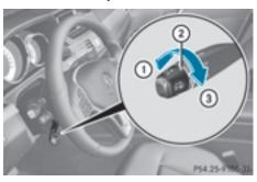
You can set the specified minimum distance for DISTRONIC PLUS by varying the time span between one and two seconds. With this function, you can set the minimum distance that DISTRONIC PLUS keeps to the vehicle in front, dependent on vehicle speed. You can see this distance in the multifunction display ( $\triangleright$  page 195).
