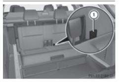
Pull the seat cushion upwards by tab ① and fold it back into its original position until it engages.
