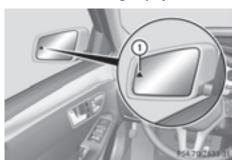
1 Yellow indicator lamp/red warning lamp Blind Spot Assist is not active at speeds below approximately 20 mph (30 km/h). Vehicles in the monitoring range are then not indicated. When Blind Spot Assist is activated, indicator lamp (1) in the exterior mirrors lights up yellow at speeds of up to 20 mph (30 km/h). At speeds above 20 mph (30 km/h), the indicator lamp goes out and Blind Spot Assist is operational.
