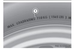
Maximum tire load ① is the maximum permissible weight for which the tire is approved. Do not overload the tires by exceeding the specified load limit. The maximum permissi-
