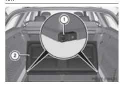
You must remove the seat cushion if you wish to lift the cargo compartment floor, e.g. if the vehicle has a flat tire.
