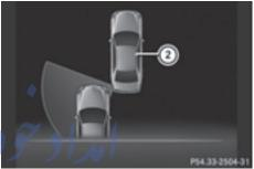
If a course-correcting brake application occurs, red warning lamp (1) flashes in the exterior mirror and a dual warning tone sounds. In addition, display (2) appears in the multifunction display underlining the danger of a side collision.
