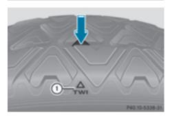
Bar indicator (1) for tread wear is integrated into the tire tread.
