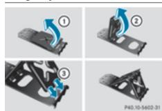
If your vehicle is equipped with a wheel chock, it can be found in the tire-change tool kit (> page 344).
