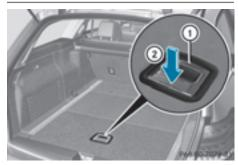
The parts of the EASY-PACK load-securing kit are contained beneath the EASY-PACK folding floor. Beneath the insert, you will find, for example, the TIREFIT kit or the emergency spare wheel and the vehicle tool kit.
