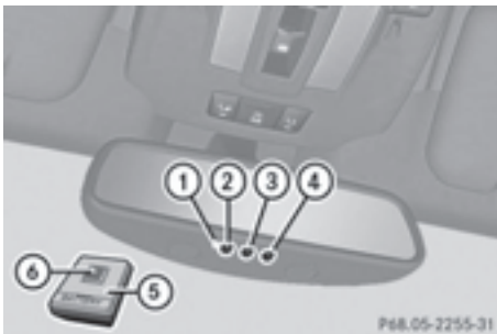
Integrated remote control in the rear-view mirror
