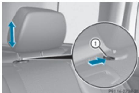
Once the head restraint is fully lowered, press release catch ①.
