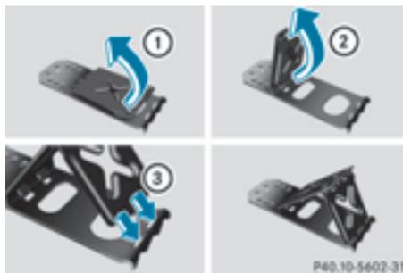
If your vehicle is equipped with a wheel chock, it can be found in the tire-change tool kit (▷ page 314).
