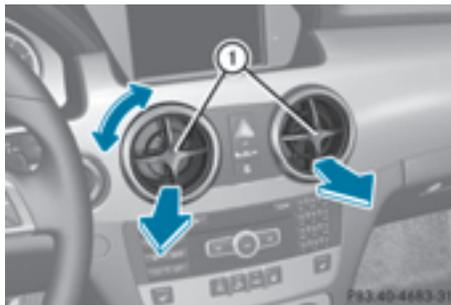
► **To open the center air vents:** turn the adjuster in one of center air vents ① to the left.
