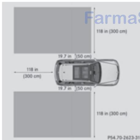
Active Blind Spot Assist monitors the area up to 10 ft (3 m) behind your vehicle and directly next to your vehicle, as shown in the diagram. For this purpose, Active Blind Spot Assist uses radar sensors in the rear bumper.
