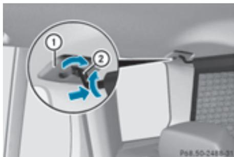
Cargo net installed behind the C-pillar
