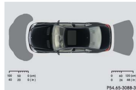
① Sensors in the front bumper (Only visible without DISTRONIC Plus*)
