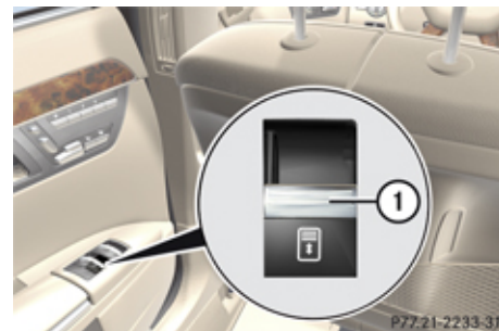
Rear door control panel
