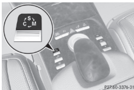
Program mode selector switch on AMG vehicles
