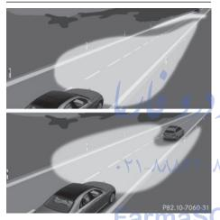
With Adaptive Highbeam Assist Plus, you can automatically switch between low-beam, partial high-beam and high-beam headlamps. Partial high-beam is a form of illumination whereby the high-beam is directed past other road users. Other road users are kept out of the high-beam. This prevents glare. When there is a vehicle in front, for example, the high-beam headlamps illuminate the areas to its right and left, and the vehicle in front is illuminated by the low-beam headlamps.
