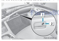
The glove box can only be locked and unlocked using the mechanical key.
