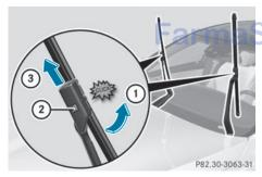
► To bring the wiper blade into position to be removed: hold the wiper arm firmly with one hand. With the other hand, turn
