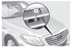
Camera lens (1) is cleaned at regular intervals by operating the windshield washer system.
