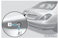
► Turn the mechanical key counter-clockwise as far as it will go from position 1 to position 2.
