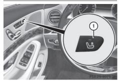
▶ To select the front-passenger seat: press button (1) repeatedly until the indicator lamp in the button lights up.
