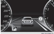
If a course-correcting brake application occurs, red warning lamp ① flashes in the exterior mirror and a dual warning tone sounds. In addition, display ② underlining the danger of a side collision appears in the multifunction display.
