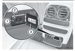
The 115 V socket is in the center console in the rear compartment on vehicles with a rear bench seat or electrically adjustable rear seats.
