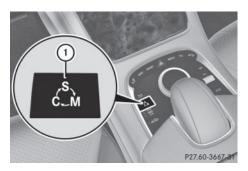
▶ AMG vehicles: press program selector button ① repeatedly until the letter of the desired drive program appears in the multifunction display.
