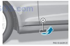
► AMG vehicles and vehicles with AMG equipment: fold cover ④ upwards.
