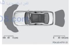
The sensors must be free from dirt, ice or slush. They can otherwise not function correctly. Clean the sensors regularly, taking care not to scratch or damage them (> page 358).
