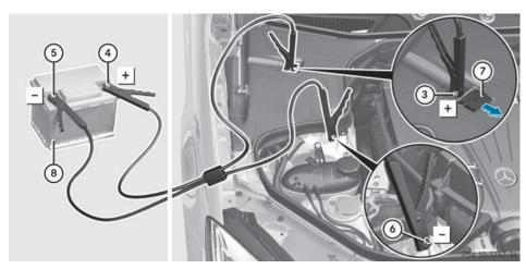
Position number (8) identifies the charged battery of the other vehicle or an equivalent jump-starting device.
