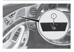
For vehicles equipped with the Warmth Comfort package: the armrest in the door and the rear armrest or the rear-compartment center console can also be heated when you switch on the seat heating of one of the front or rear seats. This can be set with COMAND (see the separate operating instructions).
