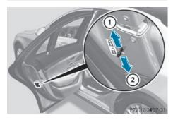
You secure each door individually with the child-proof locks on the rear doors. A door secured with a child-proof lock cannot be opened from inside the vehicle. When the
