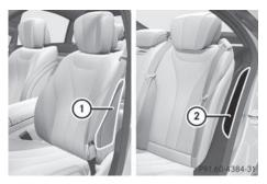
Front side impact air bags ① and rear side impact air bags ② deploy next to the outer seat cushions.
