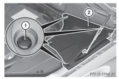
► **To open:** release retaining clamps ① and remove cover ②.
