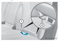
LATCH-type (ISOFIX) securing rings (2) on the rear seats are covered by a Velcro-fastened upholstered lining (1).
