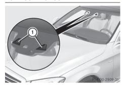
The ROAD SURFACE SCAN function monitors the road in front of the vehicle using multifunction camera ① at the top of the windshield. This function is automatically
