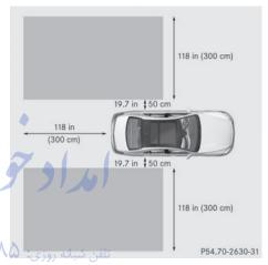
Active Blind Spot Assist monitors the area up to 10 ft (3.0 m) behind your vehicle and directly next to your vehicle, as shown in the diagram.
