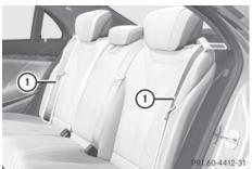
The rear seat belts are equipped with belt bags (1). These are triggered depending on the type and severity of the accident. When triggered, the belt bags open, increasing the protected area of the occupants' ribcages.
