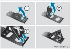
If your vehicle is equipped with a wheel chock, it can be found in the tire-change tool kit (> page 364).
