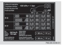
Some tire pressure tables show only the rim diameters instead of the full tire size, e.g. R18. The rim diameter is part of the tire size and can be found on the tire sidewall (⊳ page 401).
