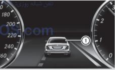
If a lane-correcting brake application occurs, display (1) appears in the multifunction display. The brake application also slightly reduces vehicle speed.
