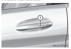
► Touch recessed sensor surface ① on the door handle until the side windows and the
