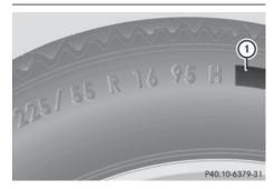
In addition to the load-bearing index, load index ① may also be imprinted on the sidewall of the tire. You will find this after the letter that identifies the speed rating (> page 401).
