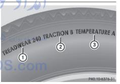
Uniform Tire Quality Grading Standards are U.S. government specifications. Their purpose is to provide drivers with uniform reliable information on tire performance data. Tire manufacturers have to grade tires using three performance factors: ① tread wear grade, ② traction grade and ③ temperature grade. These regulations do not apply to Canada. Nevertheless, all tires sold in North America are provided with the corresponding quality grading markings on the sidewall of the tire.
