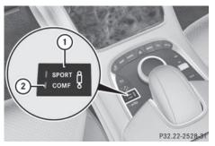
In comfort mode, the driving characteristics of your vehicle are more comfortable. Therefore, select this mode if you favor a more comfortable driving style. Select comfort mode also when driving fast on straight roads, e.g. on straight stretches of freeway.
