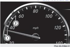
When you switch on DISTRONIC PLUS, triangle (2) shows the stored speed.
