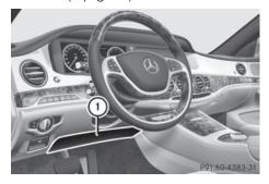
Driver's knee bag ① deploys under the steering column. The driver's knee bag is
