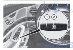
▶ To activate/deactivate: press button (2). If indicator lamp (1) is lit, operation of the rear side windows is disabled. Operation is only possible using the switches in the driver's door. If indicator lamp (1) is off, operation is possible using the switches in the rear compartment.
