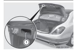
▶ Pull the trunk lid down using recess (1).
