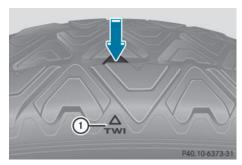
Bar indicator (1) for tread wear is integrated into the tire tread.
