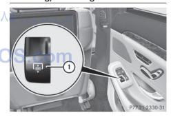
➤ To extend: pull switch ① upwards and let go.
