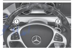
You can activate manual drive program **M** in the **E** and **S** automatic drive programs using steering wheel paddle shifters ① and ② (> page 184). In manual drive program **M**, you can briefly change gear yourself by using the steering wheel paddle shifters.
