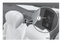
Top Tether anchorage points ① are installed in the rear compartment behind the head restraints on the parcel shelf.
