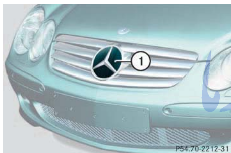
① DISTRONIC* system sensor cover
