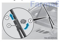
➤ To bring the wiper blade into position to be removed: hold the wiper arm firmly with one hand. With the other hand, turn the
