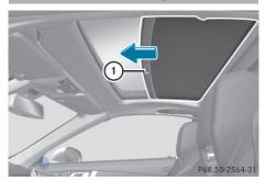
The roller sunblind protects you from excessive glare and heat caused by the sun shining through the glass roof.
