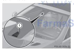
Active Lane Keeping Assist monitors the area in front of your vehicle by means of camera ① at the top of the windshield. Active Lane Keeping Assist detects lane markings on the road and warns you before you leave your lane unintentionally. If you do not react to the warning, a lane-correcting application of the brakes can bring the vehicle back into the original lane.
