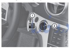
You can remove the Start/Stop button from the ignition lock and start the vehicle as normal using the SmartKey.
