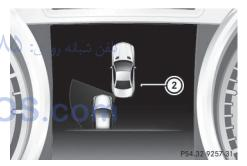
If a course-correcting brake application occurs, red warning lamp (1) flashes in the exterior mirror and a dual warning tone sounds. In addition, display (2) appears in the multifunction display.
