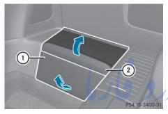
The fuse box in the rear is located on the right-hand side when viewed in the direction of travel.
