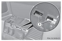
Fuses ③ are accessible through the two openings in the top of the fuse box.
