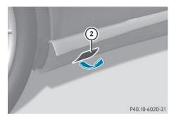
► Mercedes-AMG vehicles and vehicles with AMG equipment: fold cover ② upwards.
