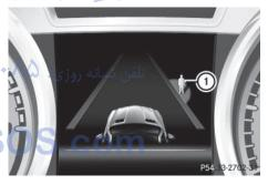
Pedestrian symbol ① in the assistance graphic indicates the status of the spotlight function. If the symbol is displayed not filled in, the function is switched on. If the symbol is displayed filled in, the conditions for the spotlight function are met.
