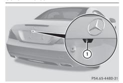
Rear view camera ① is in the trunk lid handle. Rear view camera ① is an optical parking and maneuvering aid. It shows the area behind your vehicle with guide lines in the COMAND display.
