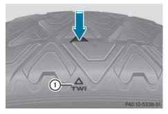
Marking (1) shows where the bar indicator for tread wear (arrow) is integrated into the tire tread.
