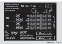
Some tire pressure tables show only the rim diameters instead of the full tire size, e.g. **R18**. The rim diameter is part of the tire size and can be found on the tire sidewall (⊳ page 260).
