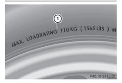
Maximum load rating ① is the maximum permissible weight for which the tire is approved.
