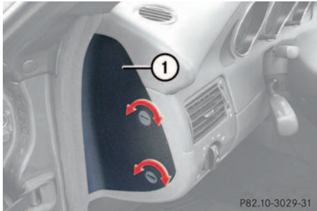
1 Auxiliary fuse box
