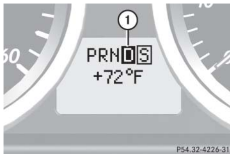
① Current gear selector lever position
