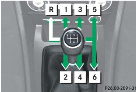
Gearshift pattern for manual transmission
